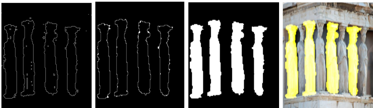
(e) Edge detection (f) Edge refinement (g) Binary Mask (h) Detection Result
