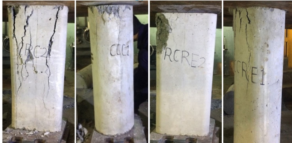
Fig. 9: Failure of Control Specimen and FECC
