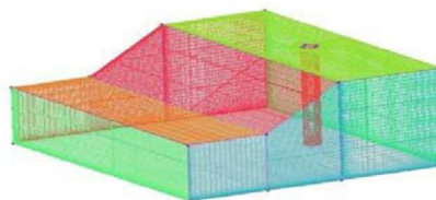
Figure.3. Meshed fuel tank used in simulation
