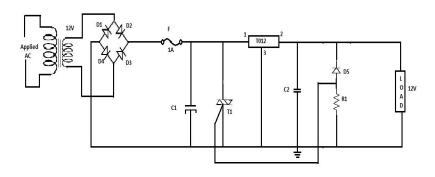
Fig. 2 Over voltage protection circuit using TRIAC as a crowbar device
