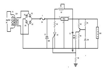
Fig. 1 Over voltage protection using SCR as a crowbar Device
