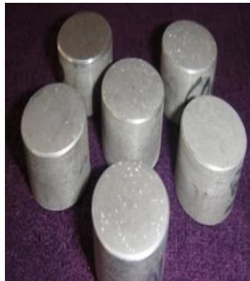
Fig.7 Hardness Test Specimens
