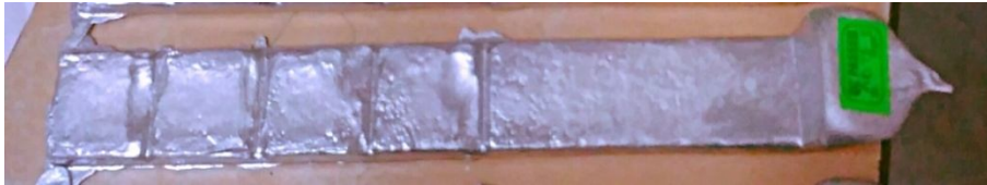
Fig.5 Specimen of A356.0 for Test of K-Mold
