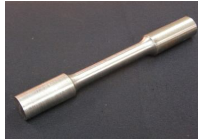
Fig.9 Tension Test Specimen
