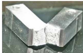
Fig.10 Toughness Test Specimen
