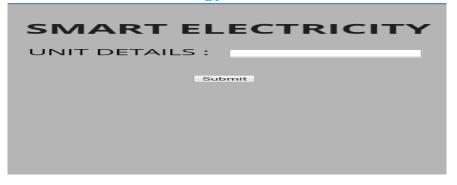
For example, if 18 watts is given in this unit details box the meter will run up to 18 watts and once the consumption reaches 19 watts the device will turn off by producing status as power exit in status bar of URL page.
