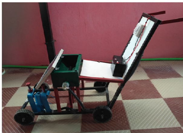
Fig 3: Model setup of a Solar powered digging and seed sowing machine
