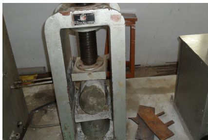
Fig 6 Test setup for Split Tensile Strength of Cylinder Fig 7 Failure mode of Cylinder
