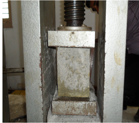
Fig 1 Specimen for Compressive Strength
