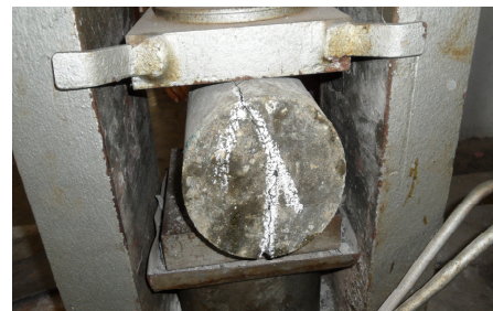
Fig 6 Test setup for Split Tensile Strength of Cylinder Fig 7 Failure mode of Cylinder
