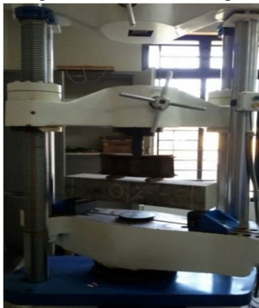
Fig. 4 Flexural Strength Test Set up
