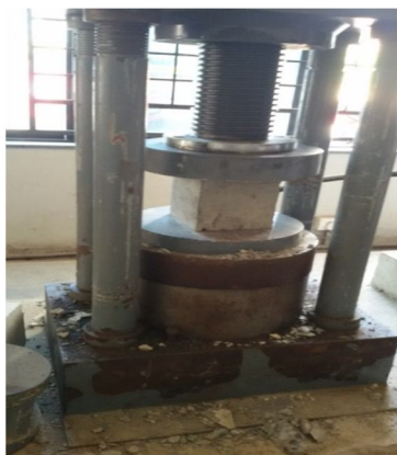
Fig.2 Compression Strength Test Set up
