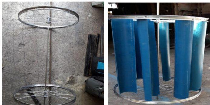
Fig 5 Mounting of shaft & Turbine blades
