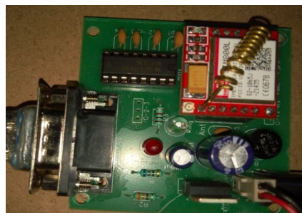
fig 5b:-DESIGNED AND FABRICATED GSM MODEM
