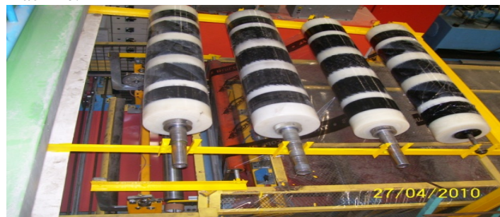
Fig. 3 Guard Film Roll Stand
