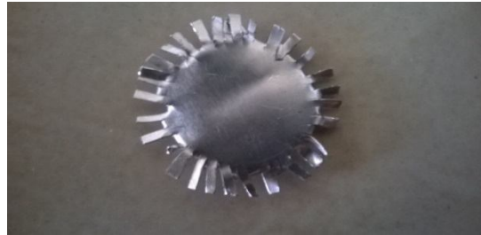
Fig 2 fabricated serrated fin with above dimensions.
