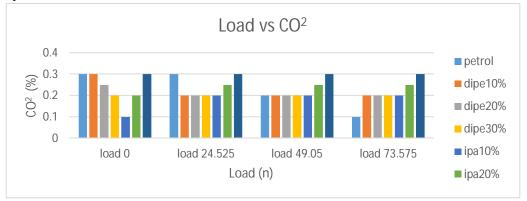
This graph shows the  $CO^2$  emission of the all the samples and petrol, almost all the blends has more emission when compared to petrol and on applying maximum load the petrol has very low emission. On comparison all are mostly equal and more than petrol.
