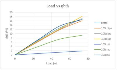
This graph shows the Break thermal efficiency of the all the samples and petrol, almost all the blends has more break thermal efficiency. On comparison the sample containing 30% of Di Iso Propyl Ether is comparatively good.
