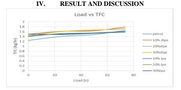
This graph shows the TFC of the all the samples and petrol, almost all the blends has more TFC. On comparison the sample containing 30% of Iso Propyl Alcohol is comparatively good.
