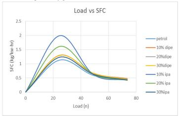
This graph shows the SFC of the all the samples and petrol, almost all the blends has less SFC. On comparison all the samples are
