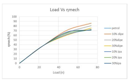
This graph shows the Mechanical efficiency of the all the samples and petrol, almost all the blends has more mechanical efficiency. On comparison the sample containing 10% of Di Iso Propyl Ether is comparatively good.
