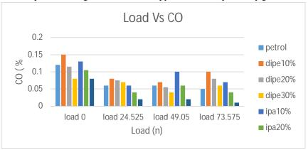
This graph shows the CO emission of the all the samples and petrol, almost all the blends have more emission on initial stage and on applying load the emission comparatively the alternative blends has very low emission. On comparison 30% of Iso Propyl Alcohol
