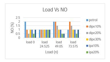
This graph shows the NO emission of the all the samples and petrol, almost all the alternative blends has very low emission. On comparison all are mostly same and less than petrol. On comparison 20% Iso Propyl Alcohol is comparatively good.
