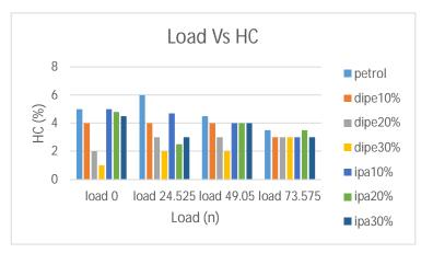
This graph shows the HC emission of the all the samples and petrol, almost all the blends has more emission on initial stage and on applying maximum load the emission comparatively the alternative blends has very low emission. On comparison all are mostly same and less than petrol.
