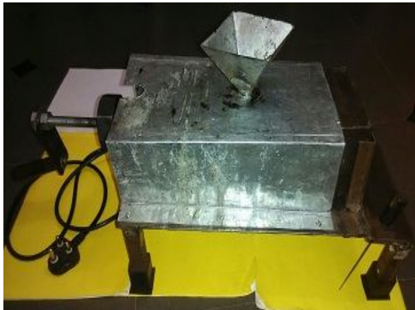
Figure3 : Design and Developed Mini Injection molding machine.
