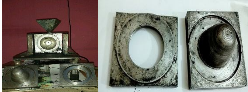
Figure2 : Mould used in injection molding machine
