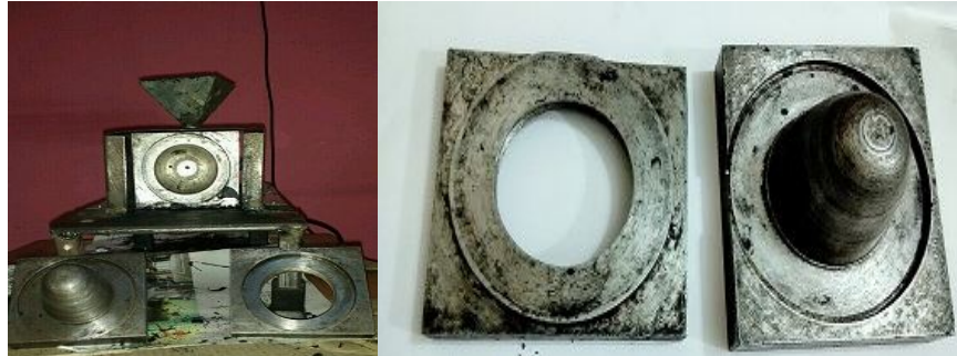
Figure2 : Mould used in injection molding machine
