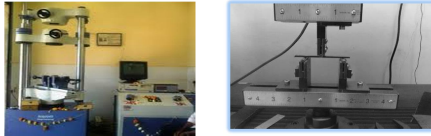
Fig. 3: UTM and 3Point Bend Test
