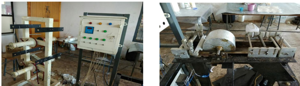
Fig. 1: Creel Stand and Resin Bath
