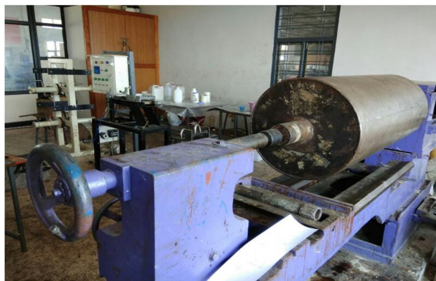
Fig. 2: Filament Winding Process
