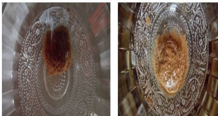
Fig. 1 Soil crumb observed after 1 hour (left) and soil crumb observed after 6 hours (right)
