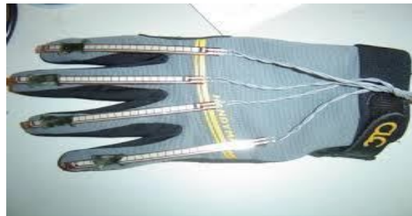
Fig 1.2 : Hand gloves with flex sensors
