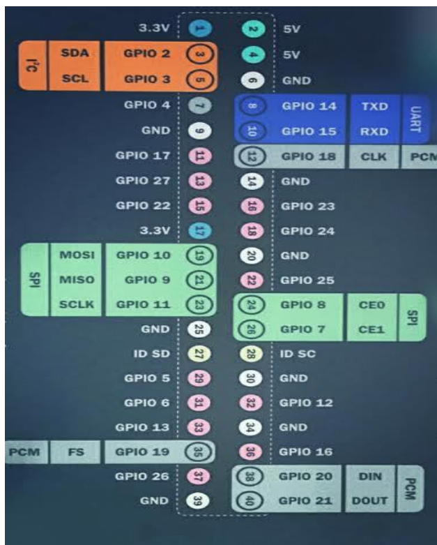
Figure 4 Pin Diagram of GPIO Pins
