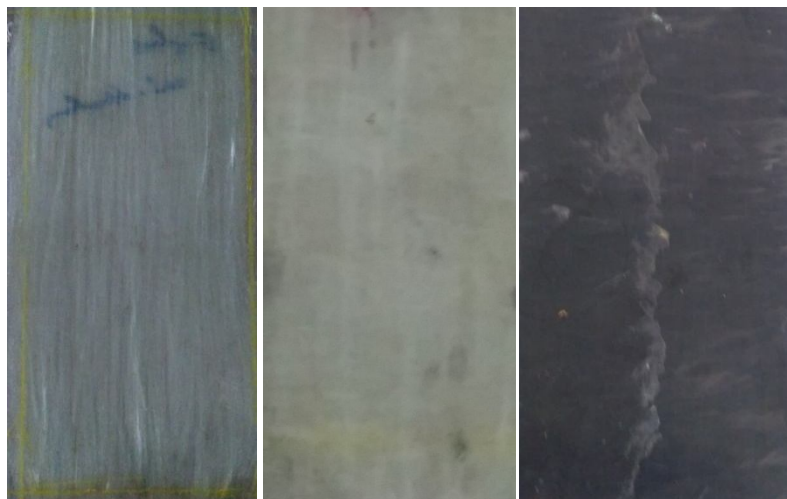
Fig1 E-glass/Epoxy Unidirectional ,Fig2 E-glass/Epoxy Biaxial , Fig3 Carbon /Epoxy Biaxial
