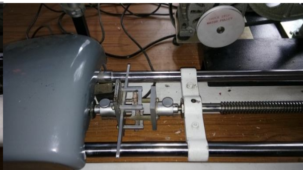
Fig.9 Sample loaded condition for flexural testing
