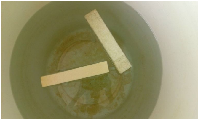
Fig 7.Specimen during water absorption test
