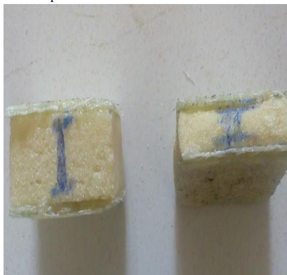
Fig 8.Specimen before & after the compression test
