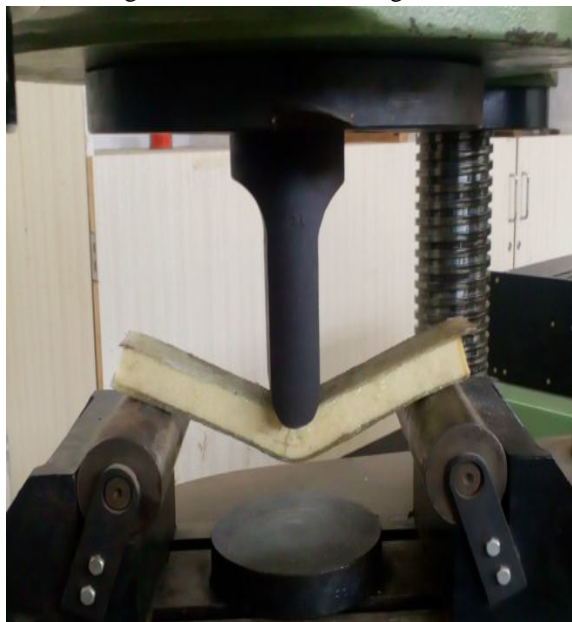
Fig 5. Specimen during bending test
