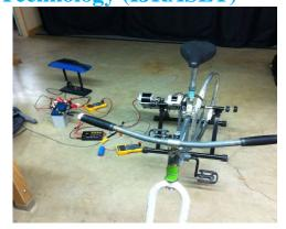
The energy which is stored in the battery will be used to run the motor and that motor with the help of a chain (free wheel) will be connected to the back wheel which helps to move the cycle with less physical efforts.
