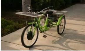
Equations of mechanics are been considered to calculate the power required to ride a bicycle, the capacity of a motor required to satisfy the power requirement can be designed. Considering the motor capacity the solar panel and the battery will be designed to
