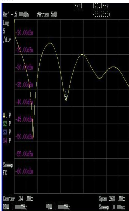
Figure(a): Resonant frequency for the second resonance is 120.1MHz
