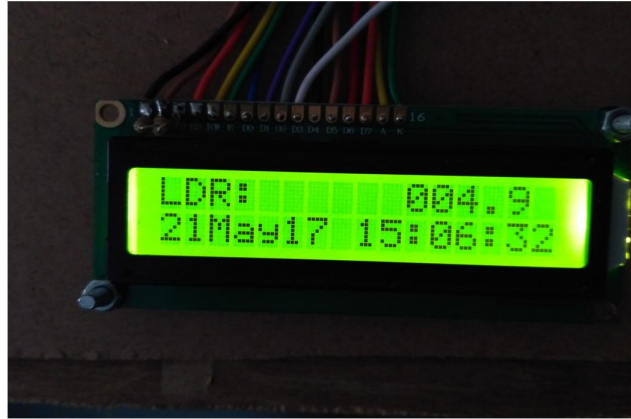
Measuring light continuously and display on LCD. Monitoring and controlling of the lumens is done.
