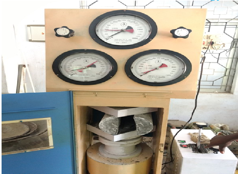
Fig.6. Testing of Cylinder for split tensile strength
