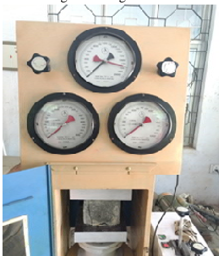
Fig.4. Testing of Cubes
