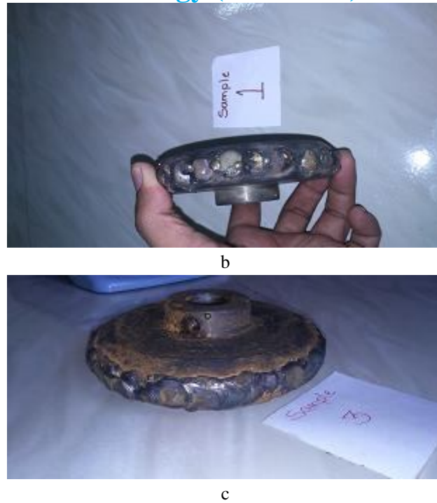
Fig. 3. Specimen's after hardfacing
