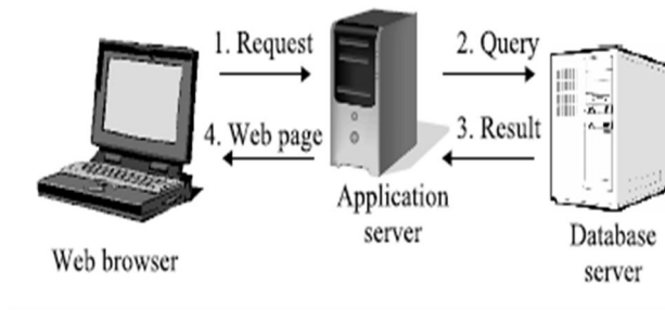
Fig. 1. Generic Request-Reply Architecture
