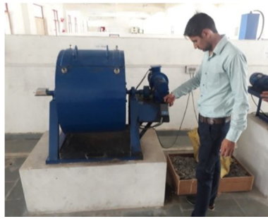
Fig. 4 Los angeles abrasion testing machine
