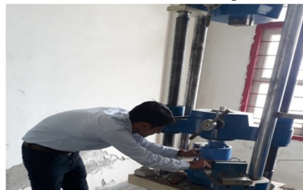
Fig. 6 Crushing strength test
