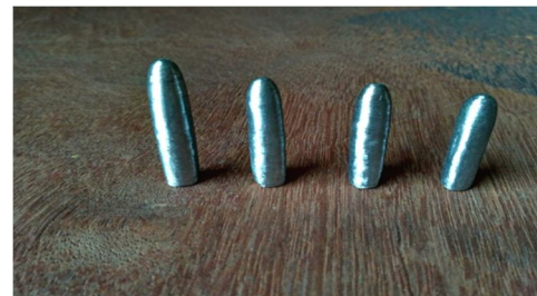
Fig 2: wear test pins extracted from hardfaced plate
