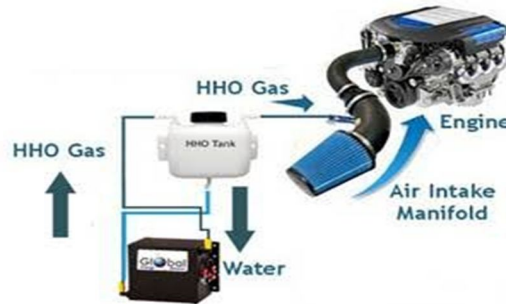
Fig: 3.2 Supply of HHO or Brown Gas to engine
