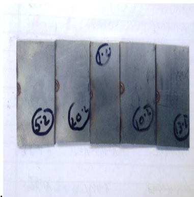
Figure 5 Vickers Microhardness test specimens
