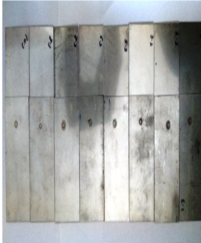
Figure 4 Tension Shear test specimens
