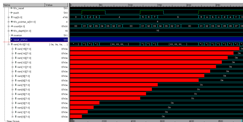
Fig. 17. Simulation result shows RAM with different data loaded at different instant of time.
