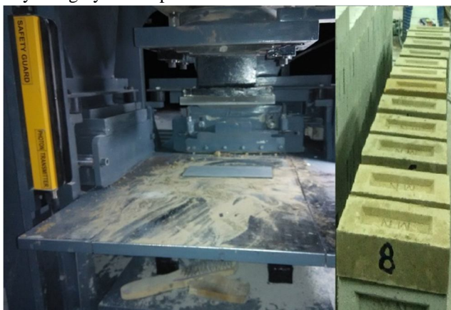
Fig.3 Casting of block in Hydraulic Compression Machine and Sample
