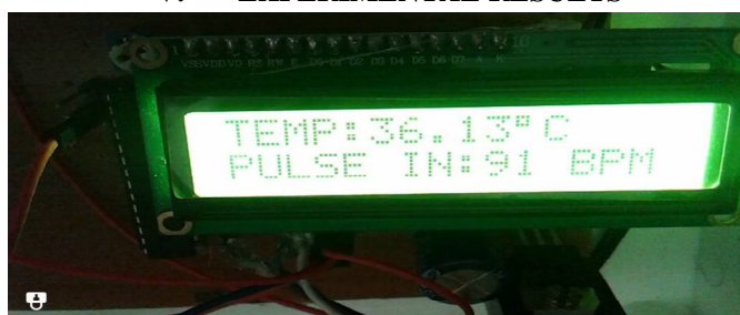
Fig. 4 Measured Body Temperature and Heart Rate displayed on LCD (Result)
