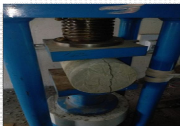
Fig 3: Shows Split Tensile Strength Test of cylinder
