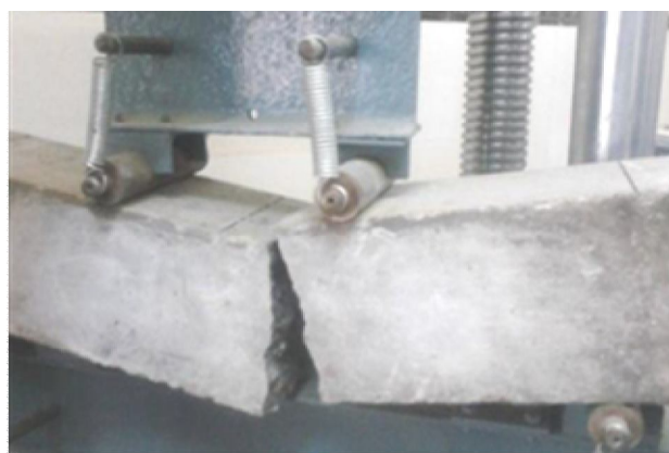
Fig 4: Shows Flexural Strength of prism
