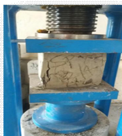
Fig 2: Shows Compressive Strength Test of Cube
