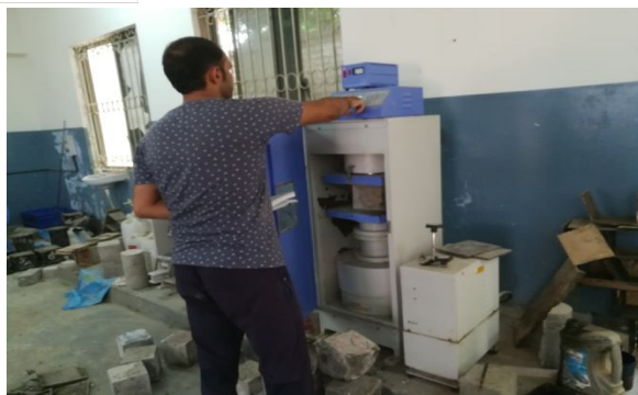
figure:4.compressive strength test of cubes.
