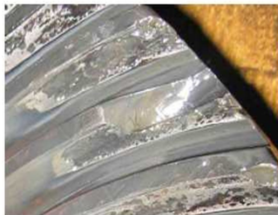
Figure 2: beach marks on gear
