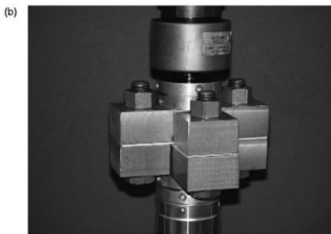
2.2 The cross tension coupon assembly drawing (a), and test fixture (b), used to conduct static tests. All dimensions are in millimeters.
