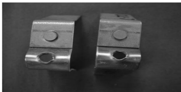
2.7 Representative image of SPR joint assemblies exhibiting rivet head pullout. Images shown are coach peel coupon assemblies after testing.
