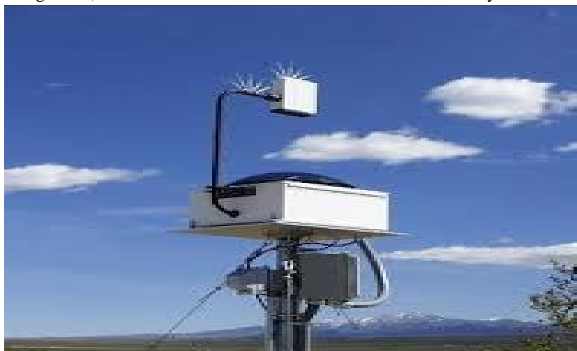
Figure.1 Total Sky Imager 440A developed by YES Inc., Ltd., USA.
