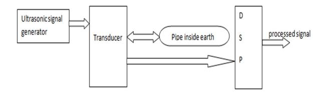
In the field of acoustics, the most common digital signal processing techniques are frequency based. Frequency-based filtering has been the chosen method of digital signal processing, because there is an analog equivalent method that was used before digital signal processing was available. Furthermore, frequency-based filtering is easily understood using basic circuit
