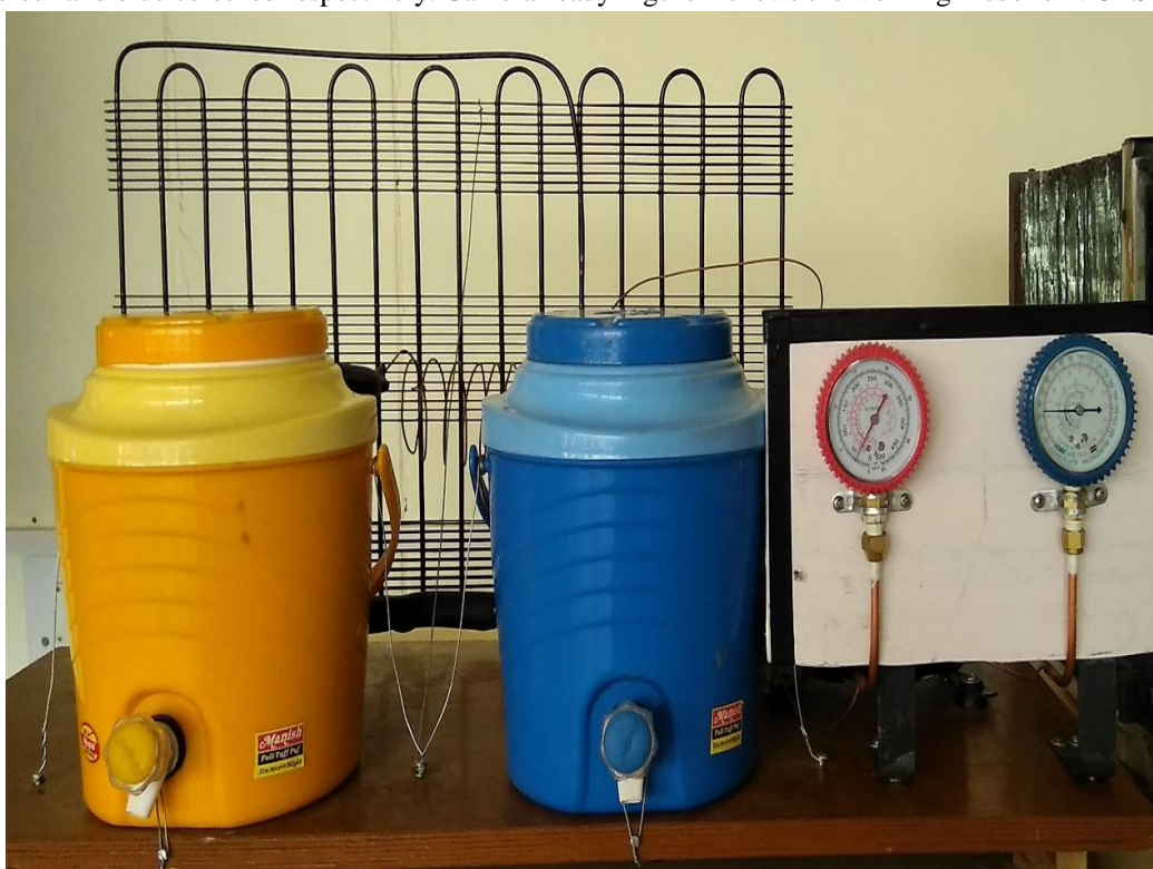
Fig. 2 Working VCRS working model (Front view)
