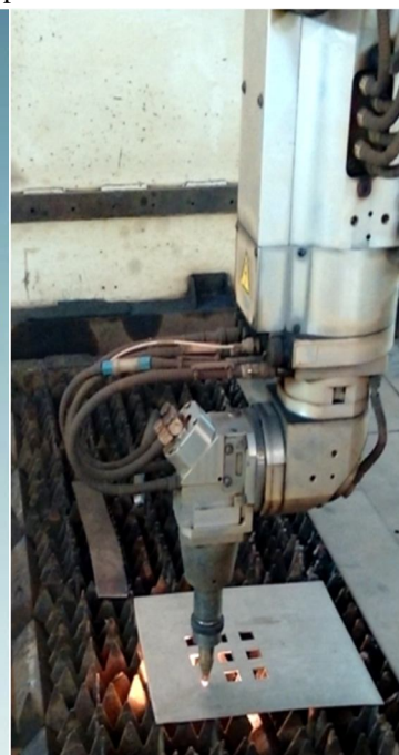
Fig. 3: CO 2 Laser Machining process
