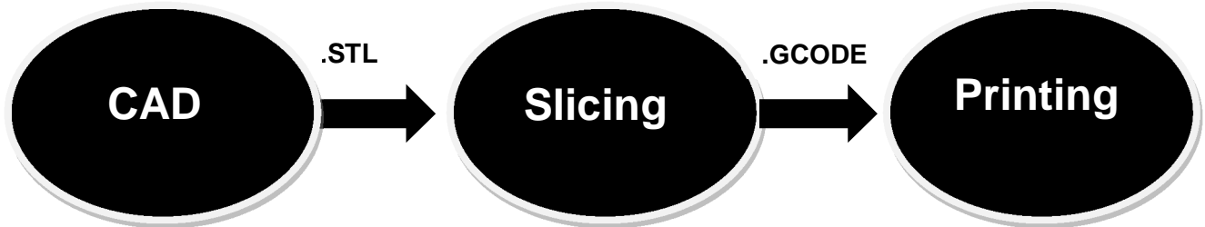
Figure 3: Different file formats throughout the printing process
