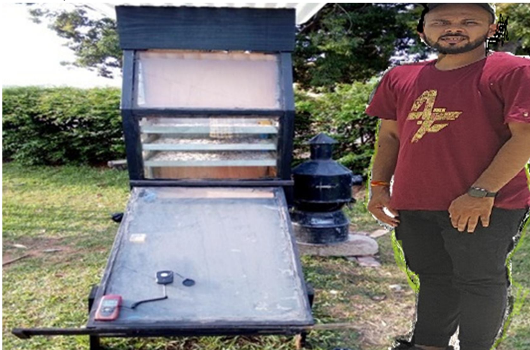
Figure 4: Isometric view of the mixed-mode solar dryer
