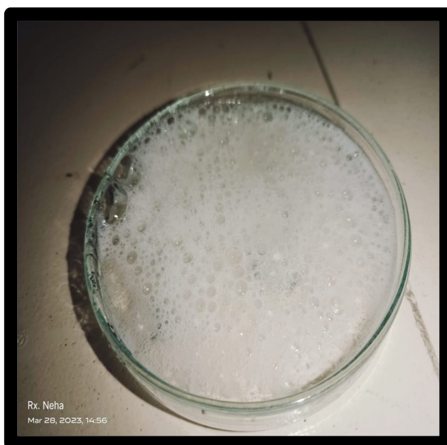
Fig.No.4: Foamability test
