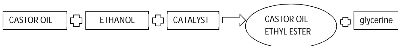
Figure4.2: Transesterification Process of Castor Oil
