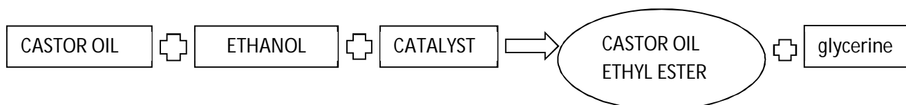
Figure4.2: Transesterification Process of Castor Oil
