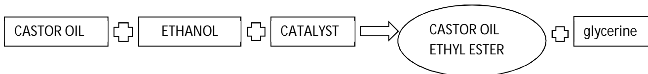
Figure4.2: Transesterification Process of Castor Oil
