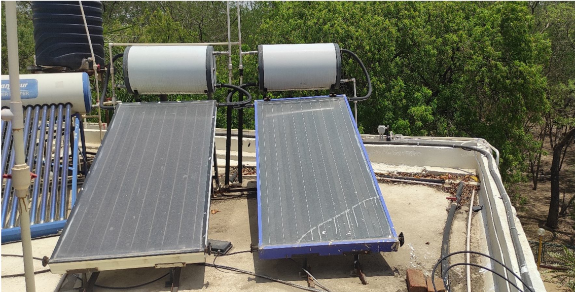
Figure 3: experiments setup water heater with glass cover.
