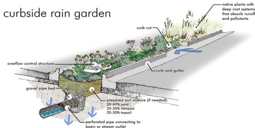
Diagram of the stormwater capture function of a bioswale, with delivery to an outlet Source
