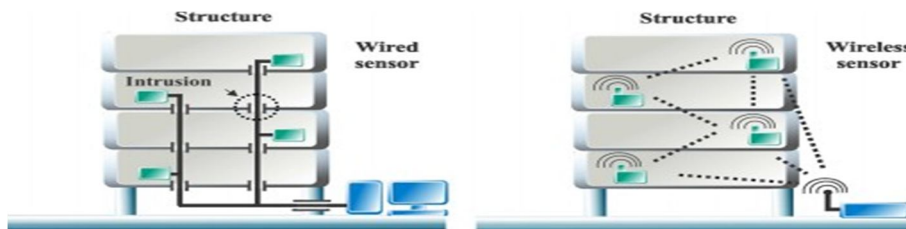
Figure 2.2: (a) Wired Sensor Network (b) Wireless Sensor Network
