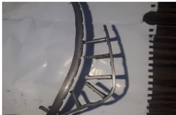
Fig.4 Failed gearbox of stand no 16 Fig.5 Broken cage bar of input shaft bearing of stand no 16-gearbox
