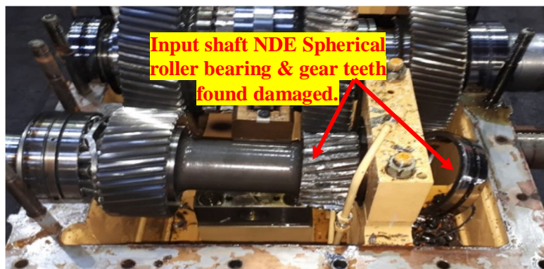
Fig.6 Failed gearbox of stand no 15
